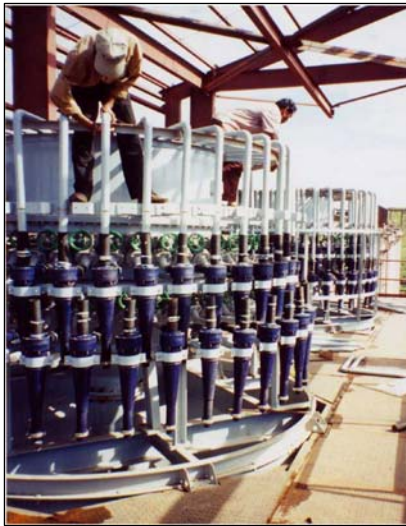
Batteries de 80 Hydrocyclones HC 100 Clusters of 80 Hydrocyclones HC 100
