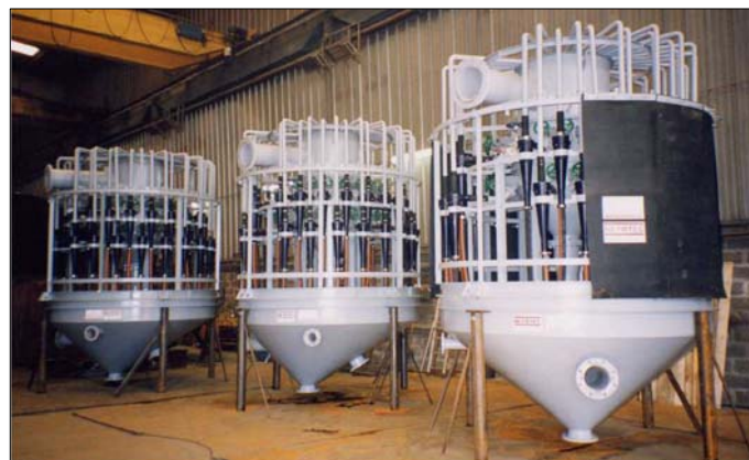
Batteries de 40 Hydrocyclones HC 100 Clusters of 40 Hydrocyclones HC 100
